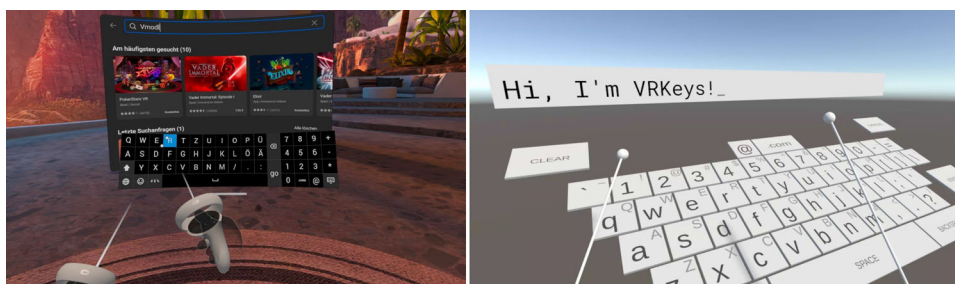
Fig. 6 Examples of VR keyboards: The Meta Quest 2's Laser pointer-style keyboard (left) and the drum-style keyboard VRKeys (right) [46]
